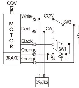
※The direction of motor rotation is as viewed from the front shaft end of the motor
